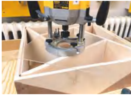
▲ Pic.30 ... and for the mirror rebate I used a hand router. I made a bigger base for the router out of some scrap Perspex. With a template for the mirror, I went to have some glass cut
